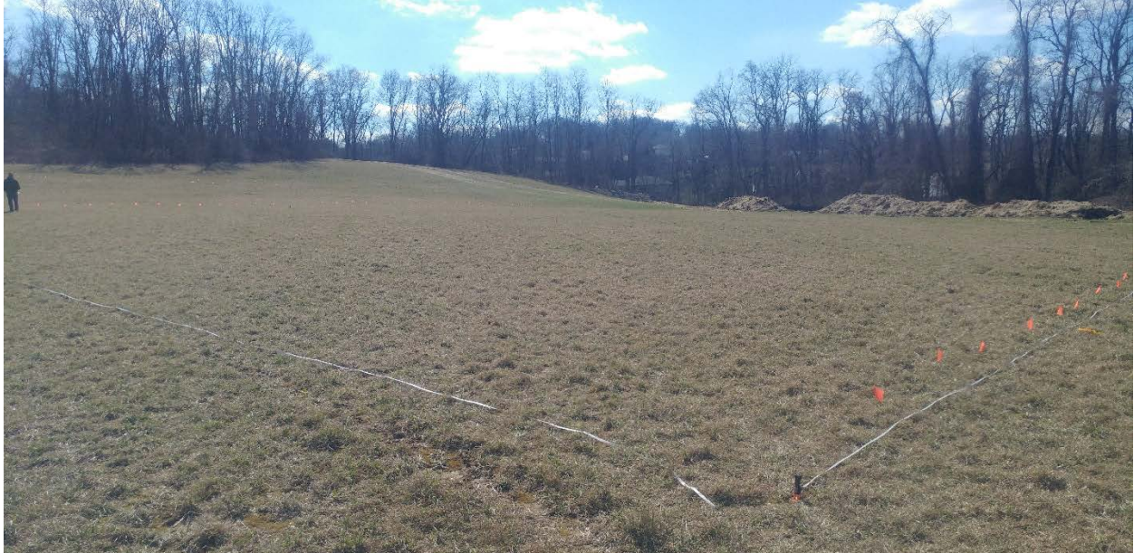
Figure 15. Photograph facing south (uphill) on the Wiest block. Image shows the layout of the Wiest 80x40mx1m grid from the NE corner of the grid. Orange flags were used to mark the north and south end points of the grid, as well as the 40m center line on each transect. Note this grid lies entirely west of the plowed area where the latest archeological test trenches were dug. The second 1m grid was installed in the uphill area visible in this image.
