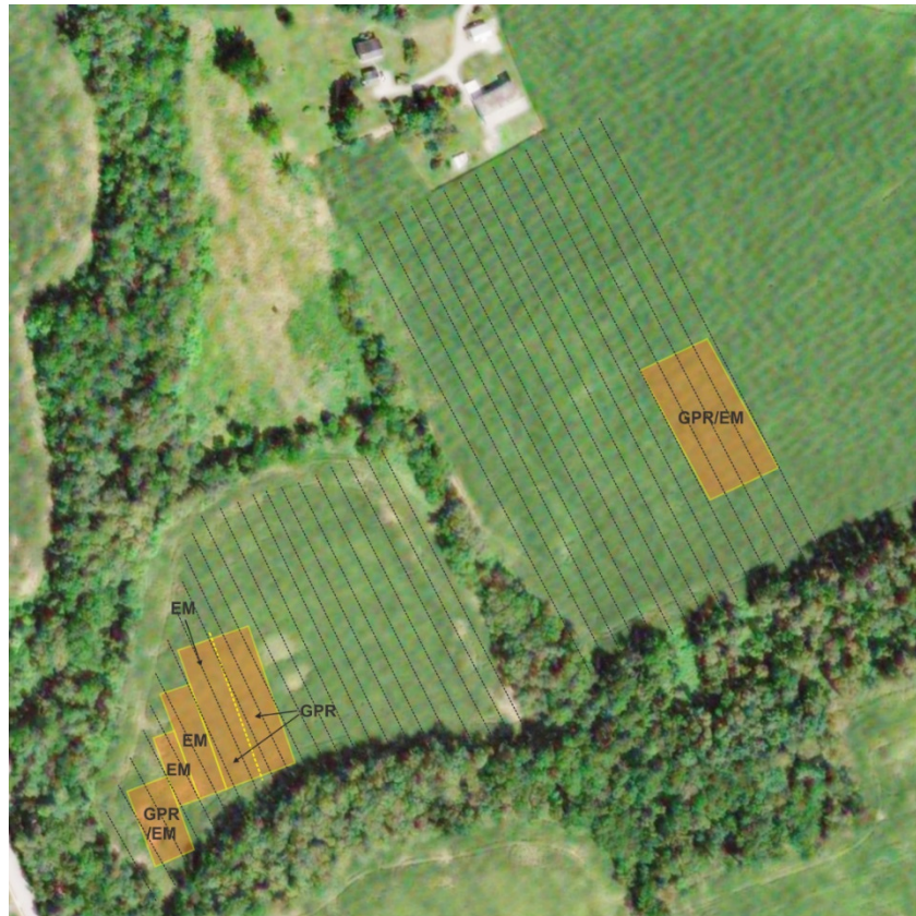
Figure 17. Overview map that shows all grids for the survey. 10m grids shown as lines, 1m grids shown as polygons.
