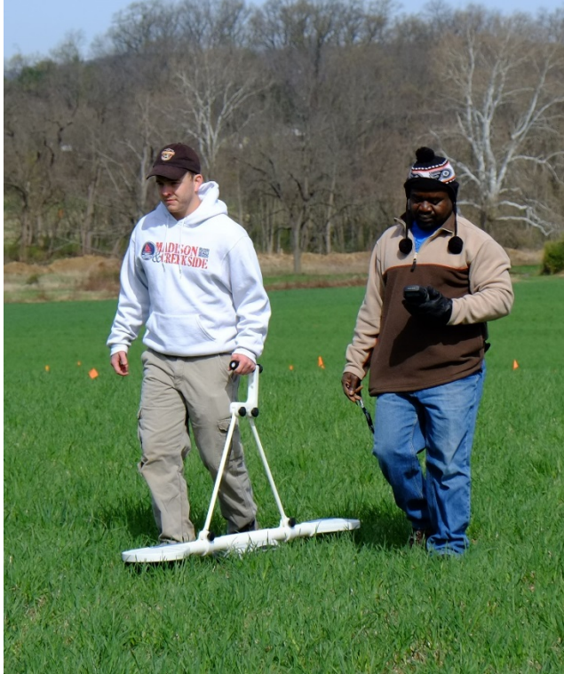
Figure 25. Data collection using the GSSI EMP Profiler unit.
