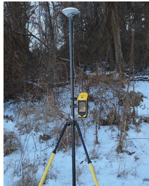
Figure 11. Photograph of GPS with external antenna used in this study.
