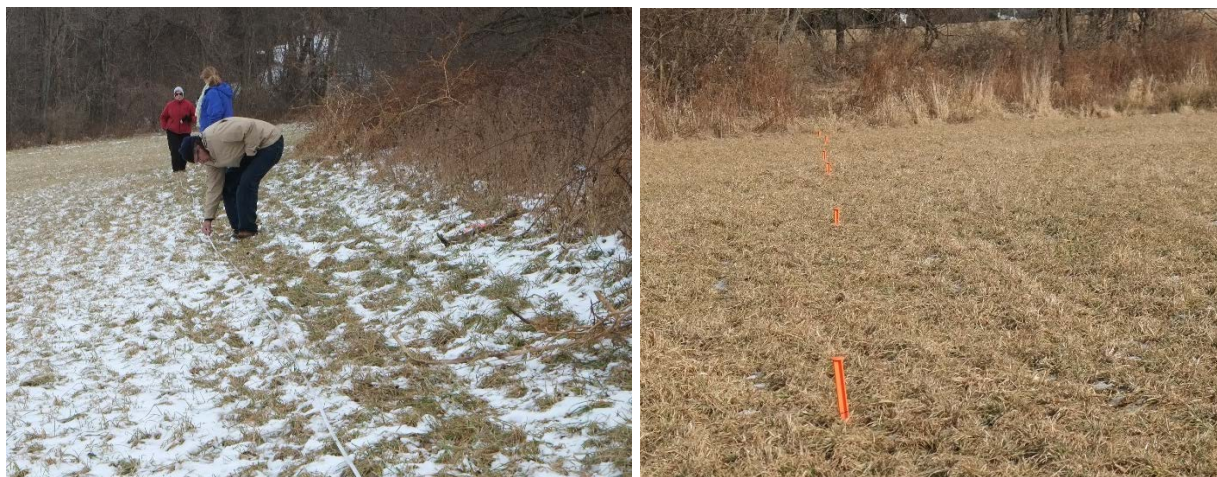
Figure 14. Volunteers assisting in set-up of the southern boundary of the Wiest block using 100m surveyor's tape (left). Surveying pins demarcate the northern boundary of the Wiest block (right). View is to the east in both cases.
