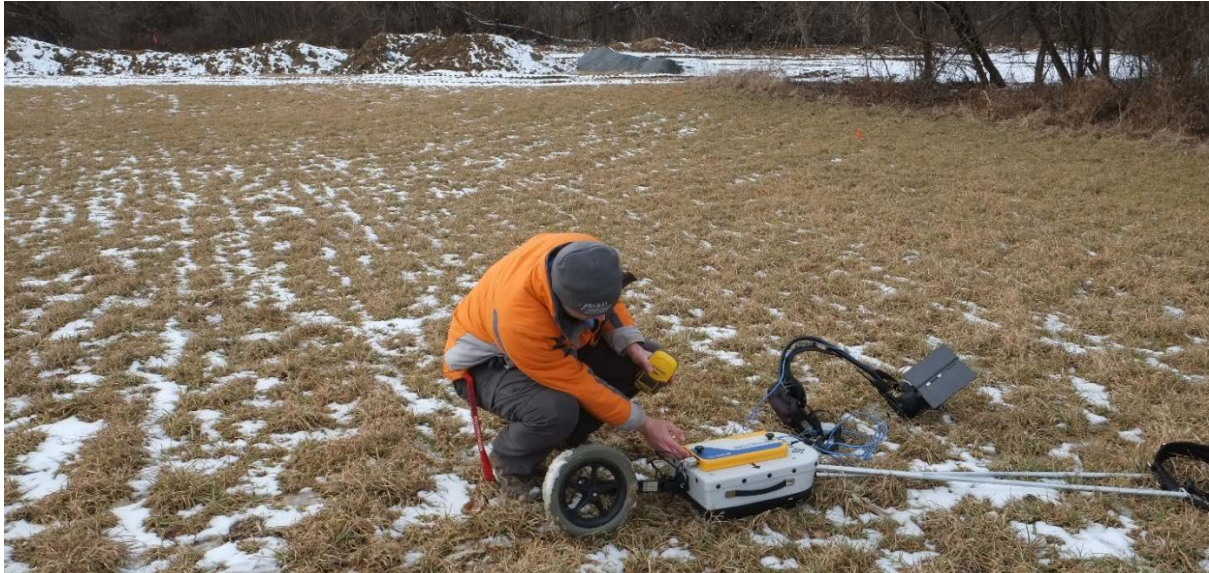
Figure 19. GPR set-up showing 500 Mhz antenna with triggering wheel attached.
