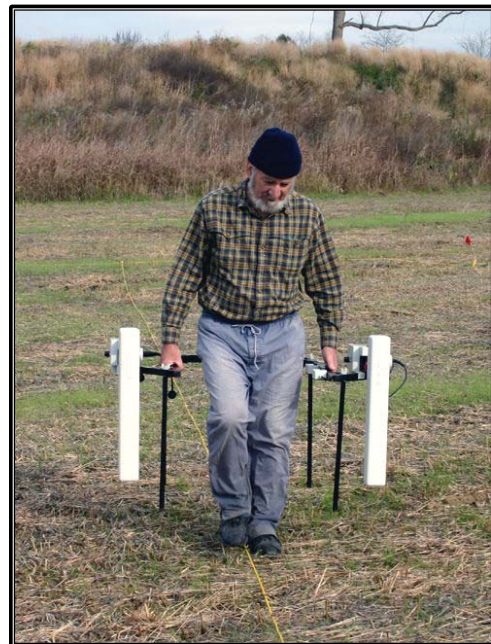
Figure 8. The Geoscan Research FM-256 Gradiometer in dual sensor configuration.
